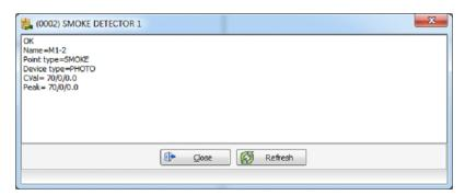
The analogical values (CVal or Peak) are captured at the alarm refresh. For run time values, the **Computer Port Protocol** can be used by typing "show 2-2-0", where 2-2-0 is the PID information corresponding to a smoke detector on our system.
