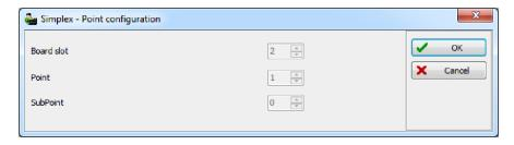
**2** - Select proper values to define the fire panel device point. Once the device is granted an address (manually or automatically from IDNet import), the user will not be allowed to change it unless the point is deleted and another one is created.
